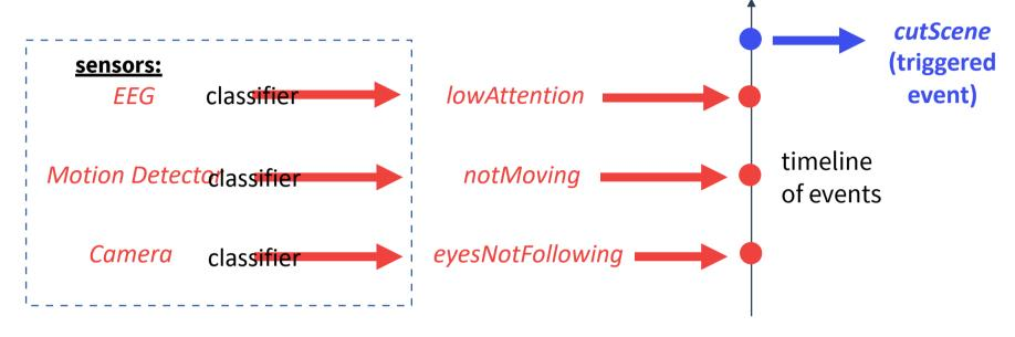
In our architecture, all the modalities are **jointly** represented on EPEC's timeline in the form of **events**. These are then reasoned about, together with the causal rules and conditional plans, to infer high-level facts about the environment (e.g., the current level of engagement) and possibly trigger other events (e.g., play a cut scene).
