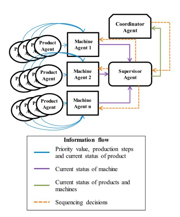
An agent-based monitoring architecture for plug and produce based manufacturing systems (Rocha AD et al)
