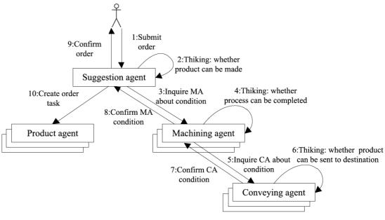
Agent-based fault tolerant framework for manufacturing process automation
